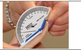
The preference for DISC is to use a **Rolyon Finger Goniometer**<sup>5, 6</sup> but we do not have a preference for the red (loose hinge) or blue (stiff hinge) variety of this goniometer.
